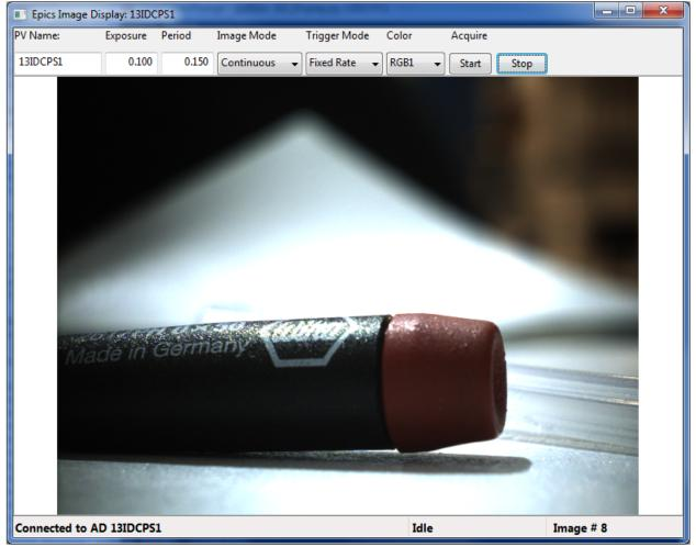
The fields and buttons on the top control several Area Detector settings, such as starting and stopping the acquisition.
